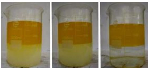
Figure 3-4 Water washing process
