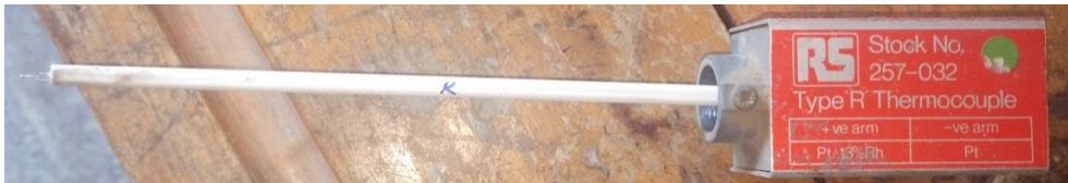
Figure 3-16 Fine type R (platinum/platinum-13% rhodium) thermocouple.
